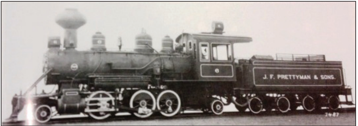
This Baldwin 2-6-2 locomotive was built for J.F. Prettyman & Sons of Summerville. It operated in the “Berkeley County Swamps.” There were no turning facilities requiring the train to run in reverse and to depend upon the cab mounted light to show the way. The image is taken from Thomas Fetter, Logging Railroads of South Carolina . 146
